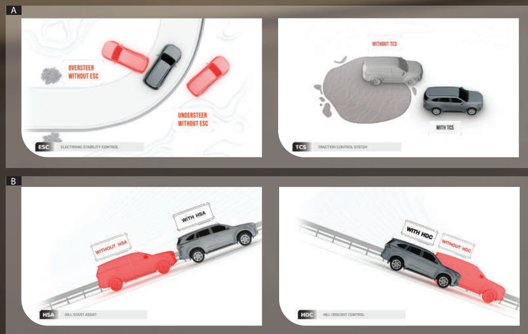
[A] Electronic Stability Control (ESC) and Traction Control System (TCS) allow for maximum road grip during acceleration and high-speed cornering.
